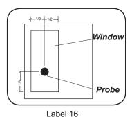
The out of balance switch is mounted on the solid part of the machine. There is a window around the probe of the out of balance switch that is mounted on the movable part of the machine.
